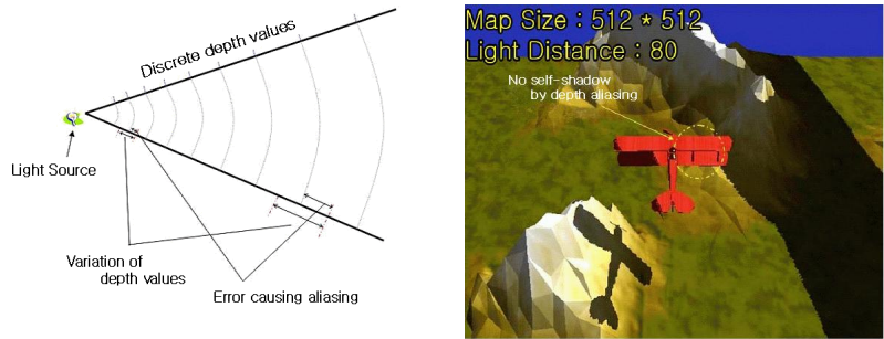
Fig. 1. (a) Why depth aliasing occurs (b) Depth aliasing makes self-shadow invisible
